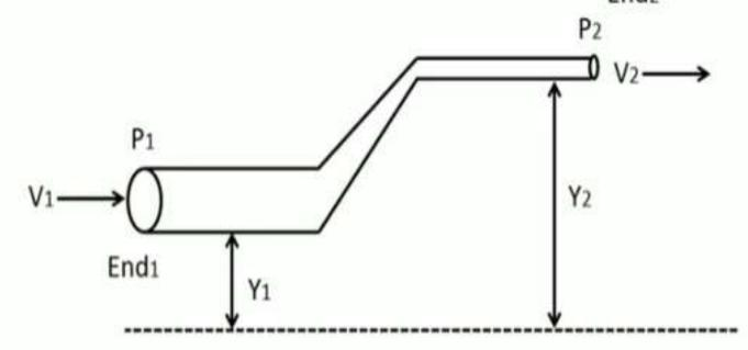
Consider a pipe as shown in figure. It can be seen that the diameter of the two ends are different. The height from the ground to each end is also different. So, the force of gravity at two ends are different.
