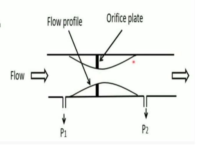
· From the figure it can be seen that there exists a permanent pressure difference (PD) in between the two sides of the orifice plate. This is the major disadvantage of using orifice plate. So, it requires more pressure to pump the liquid.
