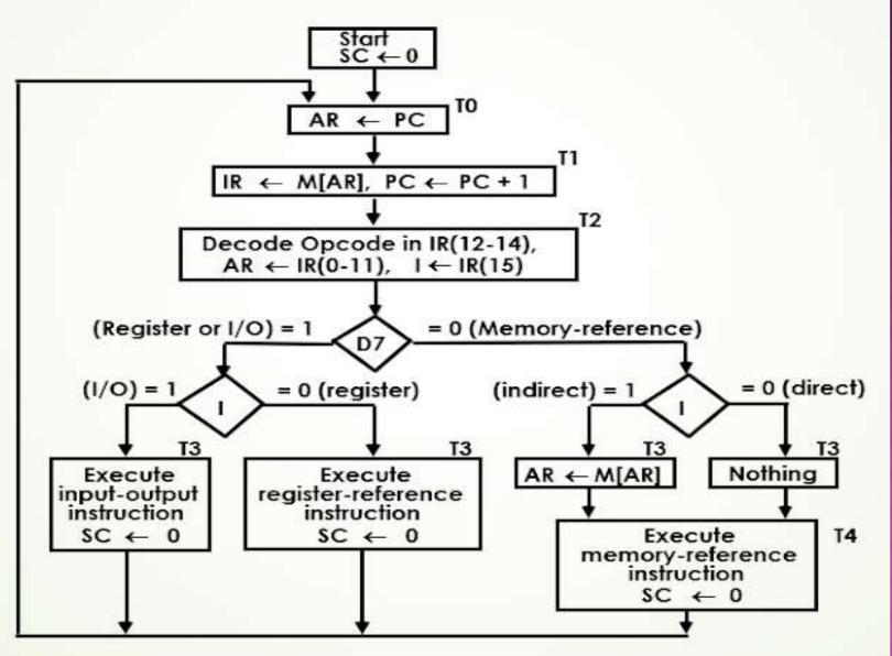
Note that the sequence counter SC is either incremented or cleared to 0 with every positive clock transition.
