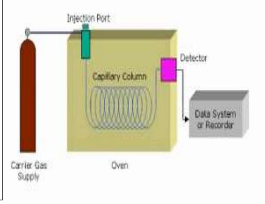
As the mobile phase (carrier gas) carries the vaporized sample through the column, separation of components occurs; due to their differential partitioning and equilibration between the stationary liquid phase and the carrier gas.
