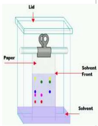
•The lower edge of the paper strip is spotted near its edge with the solution containing the components and dried
