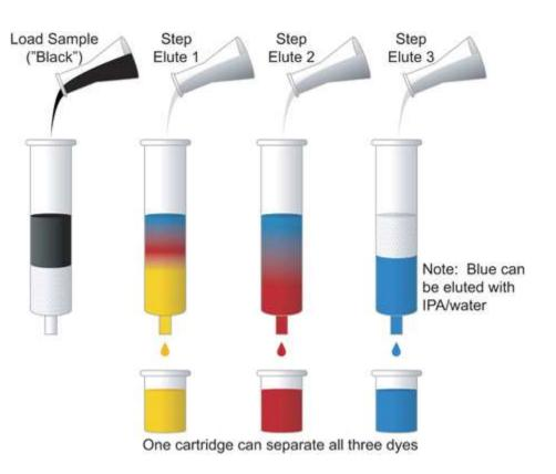
Liquid- solid adsorption chromatography is based on the selective adsorption of the sample components on an adsorbent column
