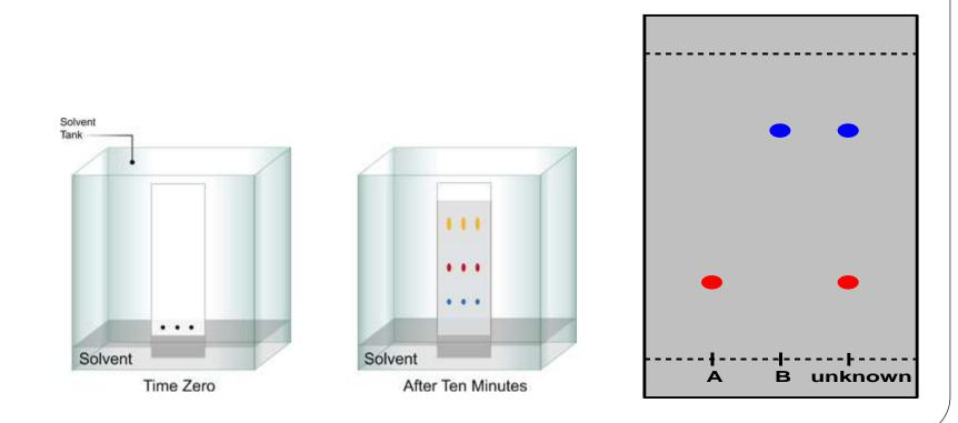
□As the mobile phase, ascends by capillary action carry the various components and yields compact spots within a few minutes.
