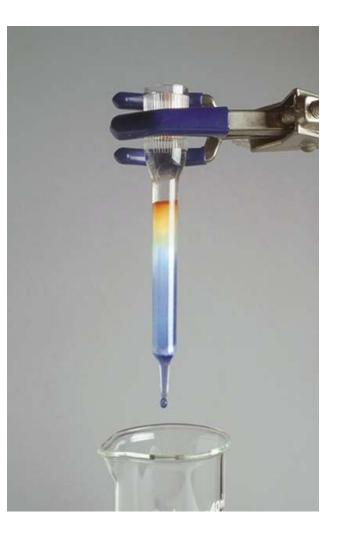
The individual components are extracted from the adsorbent by passing a suitable solvent (the same or a different one) down the column.
