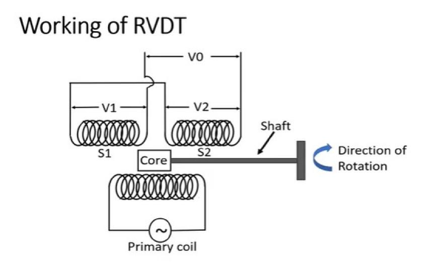
The differential output is V0 = V1 - V2
