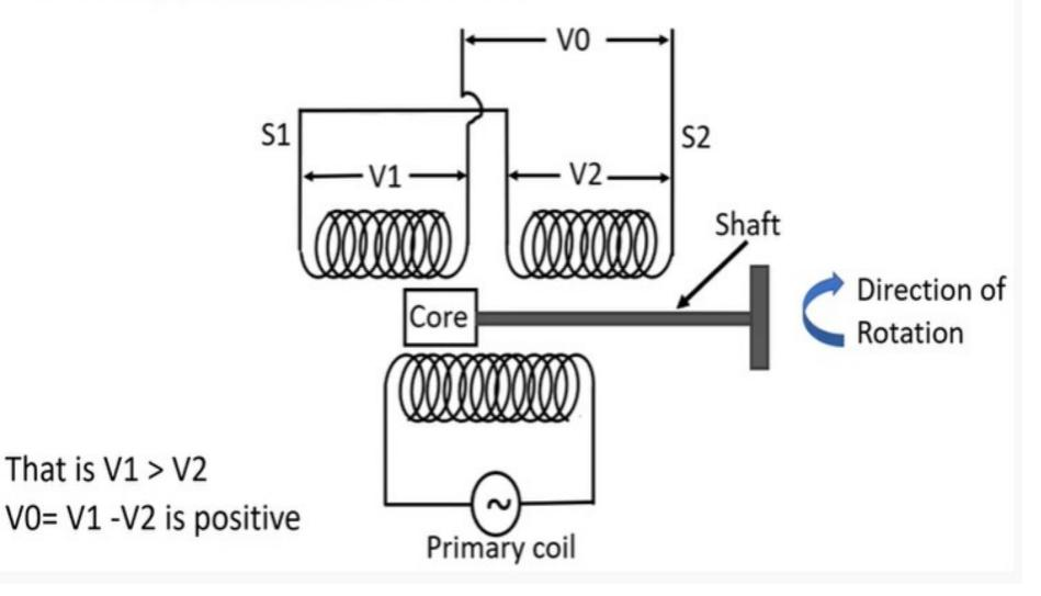
CASE 3: The core position is towards the S2 windings of the secondary (for anti-clockwise movement)
