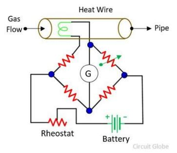
• When the wire is kept in the stream of liquid, in that case, the heat is transferred from the wire to the fluid. The heat is directly proportional to the resistance of the wire. If heat reduces, that means the resistance of wire also reduces. The Wheatstone bridge measures the variation in resistance which is equal to the flow rate of the liquid.
