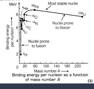
The graph has its maximum of 8.8MeV/nucleon where the mass no.is  $56.(_{26}Fe^{56}-an$  isotope of iron). This is therefore the most stable nucleus.
