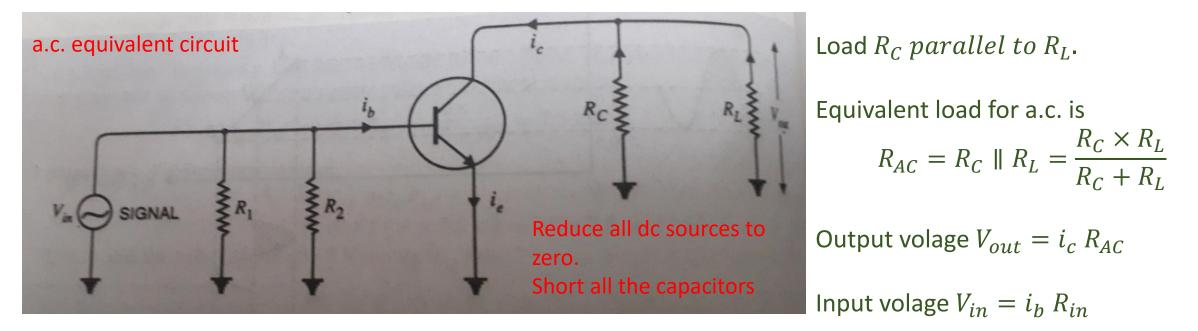
Open circuit Voltage gain
