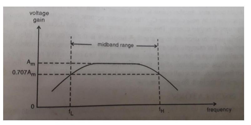
Band width of an amplifier is the difference between upper and lower cut off frequencies.
