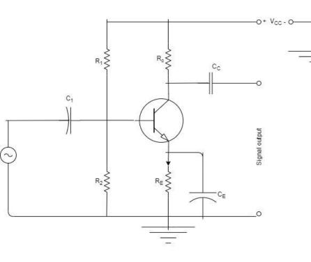
Total base current = dc base current + ac base current  $i_B = I_B + i_b$
