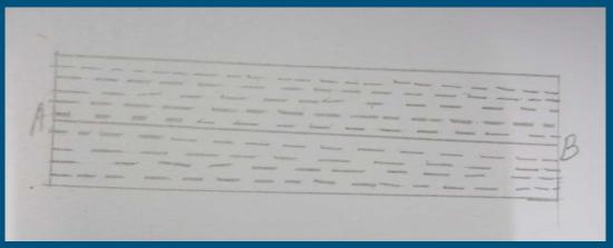
The beam is considered as made up of large no. of thin plane layers arranged parallel to each other.
