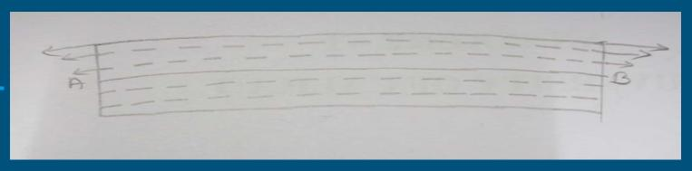
Let the beam subjected to deforming forces ,the beam bends.
