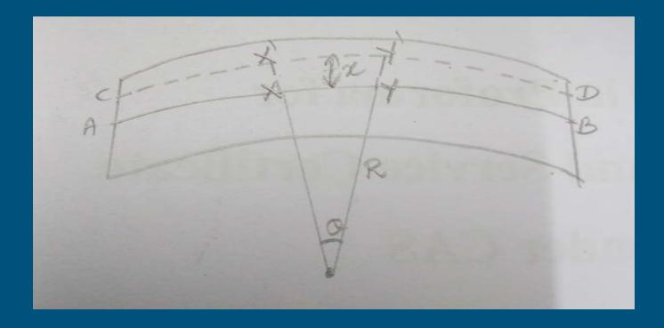
Consider the portion of a layer  $X^{I}Y^{I}$  at a distance of x above the neutral axis. The neutral axis bends to the form of a circle of radius R subtending an angle  $\Theta$  at its centre
